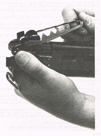
Fig. 3.—Removing the gas plug.
