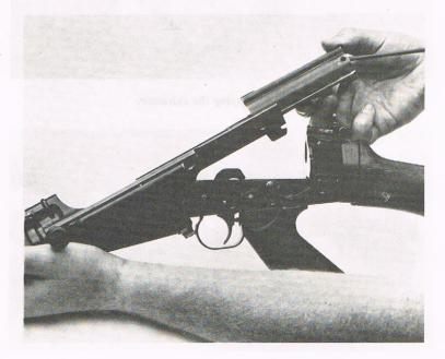
Fig. 9.—Putting back the breech block and slide.
