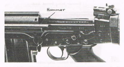
Fig. 24.—The hammer hitting the firing pin.
