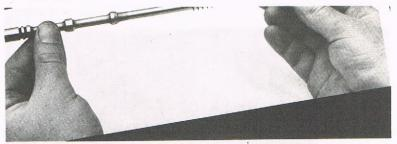
Fig. 10.—Putting the piston spring on the piston.
